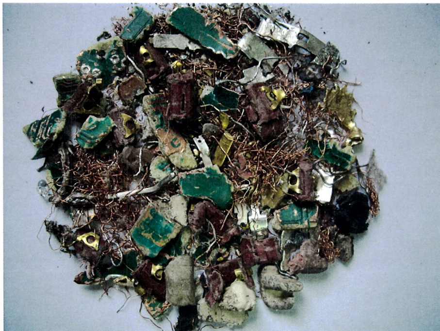
Fig.1 Material mixt: Fire Cu/Al, Placute electronice, Alama 0-5mm
