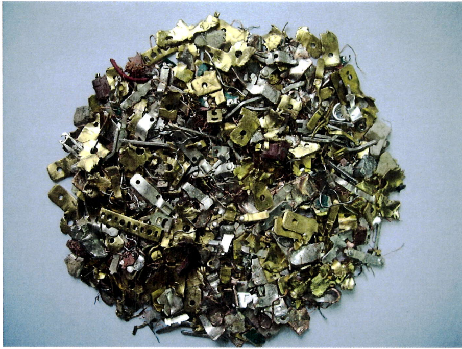
Fig.2 Material mixt – Material neferos: Alama, Cu, Al
